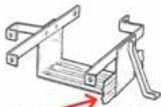
Note the extra horizontal metal plate to protect the battery from front wheels throwing water and debris.
